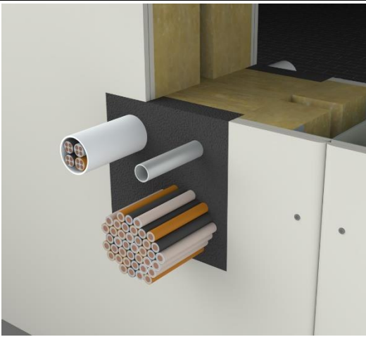
Fig.8 Electrical cable in casting pipes penetration seals in gaps: area \leq 225 cm 2 or max. 150x150mm, wall A \geq 100 mm
