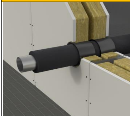
Fig. 5. Pipe in rigid wall A \geq 150 mm
